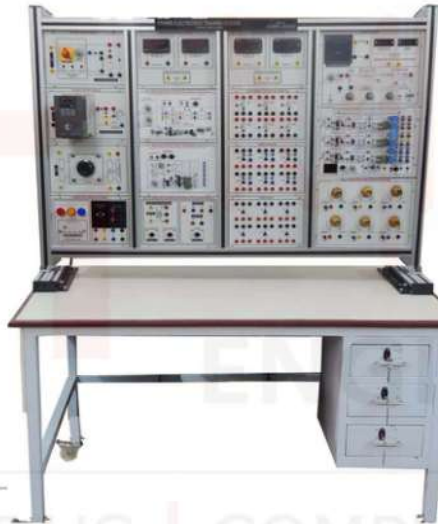
MT-E657C POWER ELECTRONIC TRAINING SYSTEM (TEST BENCH)
